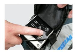
iii. Activate the press button fob to confirm that the pump is working. The **RED** light on the pump enclosure will illuminate and the sound of the pump will be heard.
