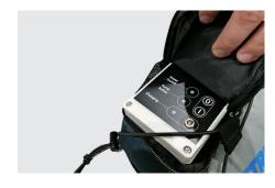
ii. Insert the battery charging plug unto the socket on the pump enclosure.
