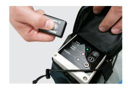
iv. Slide the pump enclosure into the back pack and zip the compartment closed.
