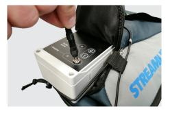
iii. Plug the charger into a 230v mains power supply and switch it on. The blue charging light on the pump enclosure will illuminate.
