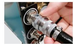
iii. Connect the **RED** hose from the waste water outlet and direct to a drain or nearby Soakaway
